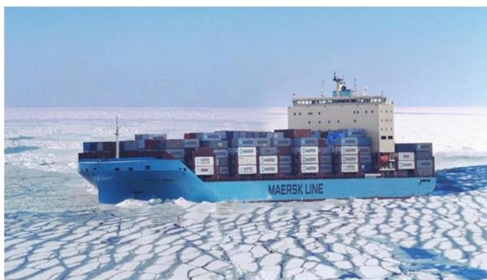
Illustration of a Maersk Arc4 ice-class container ship sailing through ice on the Northern Sea Route. (Source: Photos courtesy of Rosatomflot and Kwak Dongmin. Composition courtesy of the author.)
